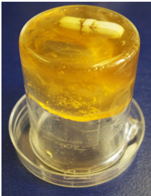
Fig. 7. Self-crosslinked modified chitosan gel produced by dissolving 6% (w/w) of the chitosan-6h in distilled water (pH \sim 5.5 ). The beaker was placed upside down showing the gel holding the stirring bar in place revealing its mechanical stability.
